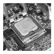
After confirming the CPU direction for correct mating, put down the CPU in the socket housing frame. Be sure to grasp on the edge of the CPU base. Note that the alignment keys are matched.
